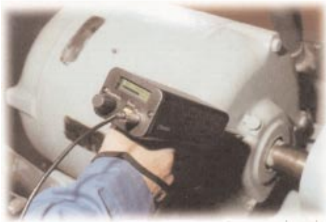
Checking grease levels using ultrasonic leak detector.
