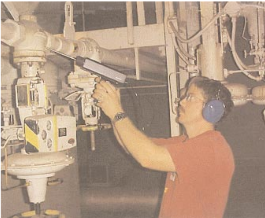
An HECO technician demonstrates ultrasonic inspection using the UE Systems Ultraprobe 9000™
