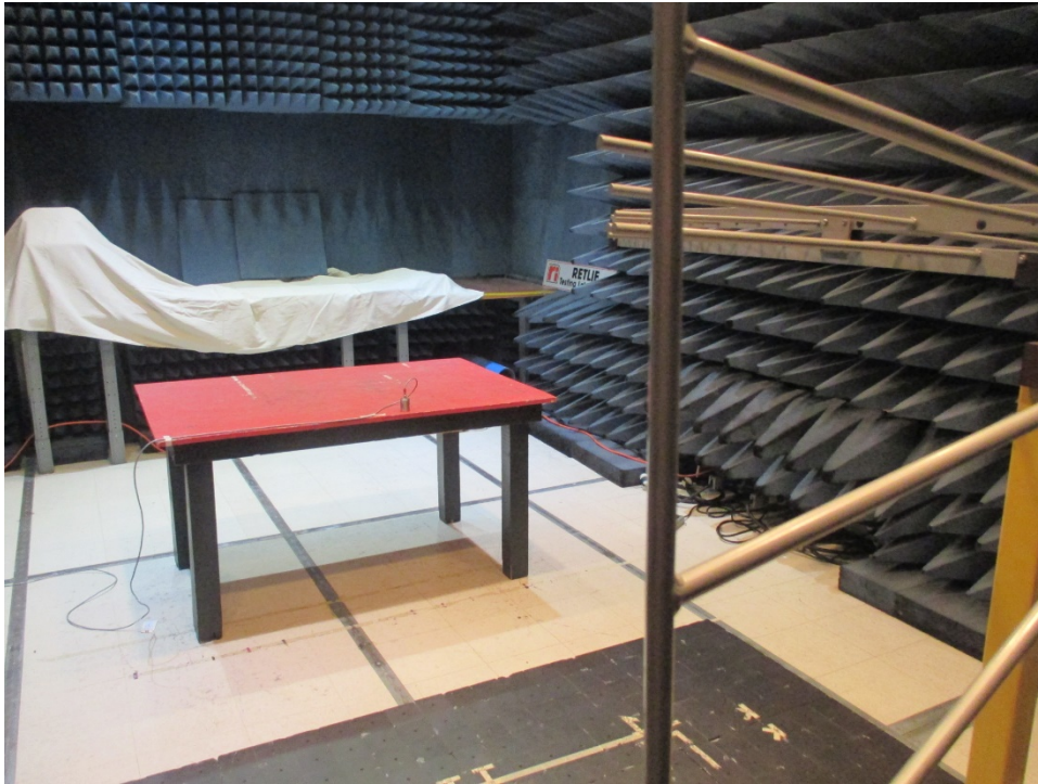
Horizontal Antenna Polarization, 80 MHz to 1 GHz, Side 2
