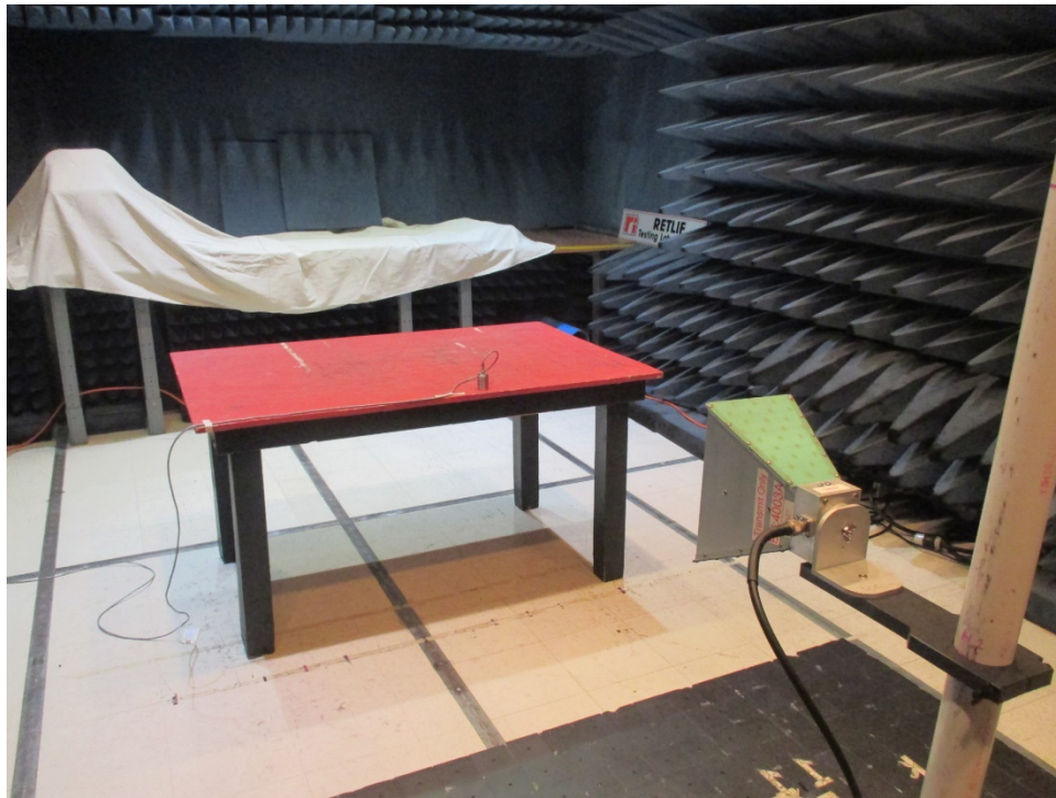
Horizontal Antenna Polarization, > 1 GHz, Side 2
