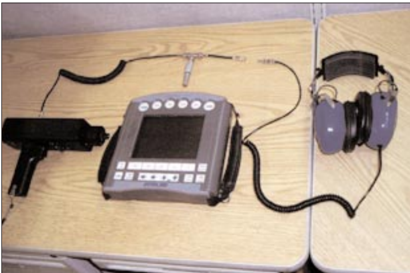
Figure 1 - Prepare a "y" cable that will plug into the detector on one end with the other end plugged into the data collector.
