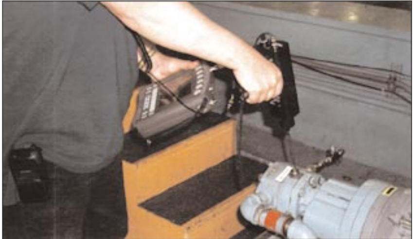
Figure 2 - For the purpose of demonstration, data is taken on a hydraulic pump for both ultrasonic as well as vibration readings.
