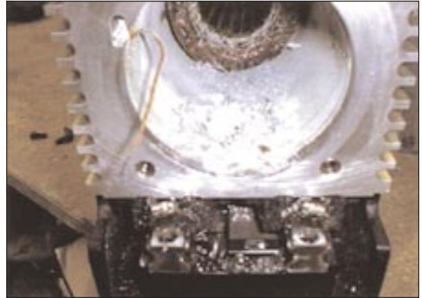
Figure 9 - View of the spindle during disassembly showing the remnants of ceramic bearing. Talk about catching them in stage 4!
