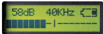
Scala calibrata in dB riconducibile a NIST
