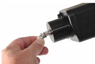
Step 3 - Connect an Ultraprobe to the box
