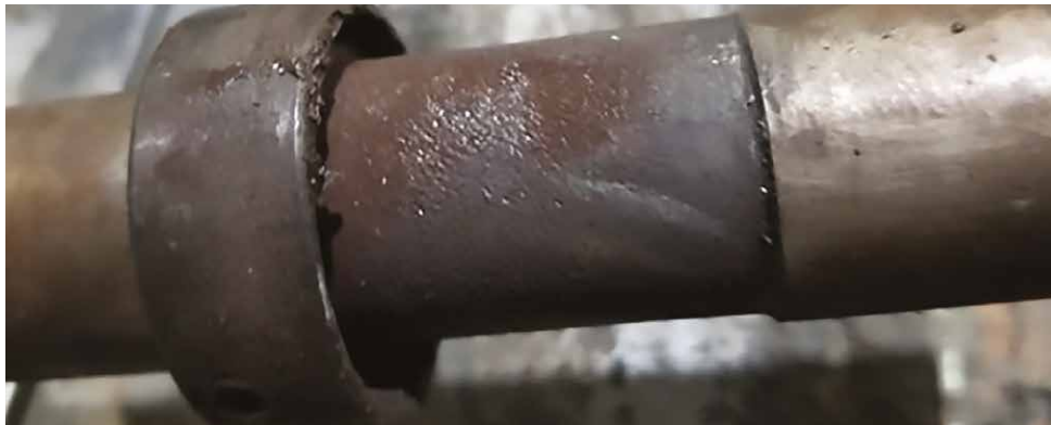
Damaged shaft from bearing failure.
